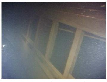
Exterior wall of passenger cabin showing window frames
